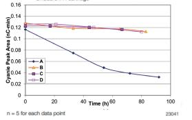
Figure 2: Effect of dissolved copper on free cyanide (10 µg/L)
