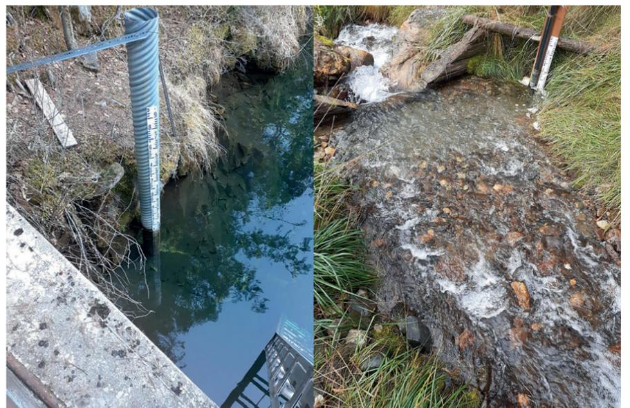
Solinst Levelloggers are Installed in PVC or Steel Pipe in Streams to Record Water Levels
