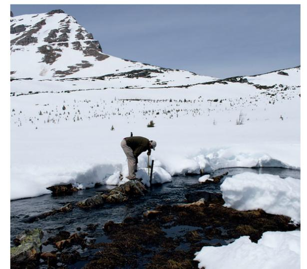
Solinst Levellogger Recording Water Levels in an Alpine Lake Stilling Well
