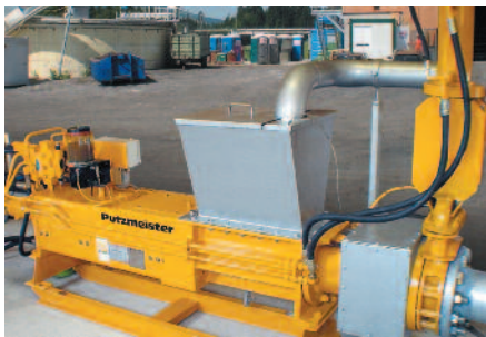
Fig. 1 The biomethanisation plant in Kössen (Austria) is using an EKO 1060 PP to convey and unwrap packaged foods that are past their expiry date.
