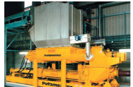
aFig. 4 In the biogas plant of Varenne-Jarcy (France), this PM high-density solid pump conveys biomass in a fermentation tank
