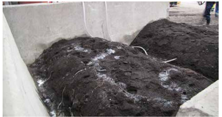
Figure 3. Three months later the fungal mycelia are growing on the surface of and inside the fungal treatment pile (fungal treatment pile in front).
