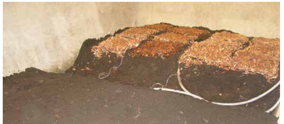
Figure 2. Fungal inoculum is set inside the soil pile in layers (fungal treatment pile behind).
