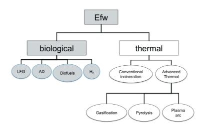
Figure 1: Energy from Waste technologies
