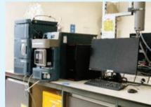
Dr Daniel Baker runs our LC-MS facility that delivers analytical testing of pharmaceuticals and other analytes using our recently installed Waters TQ-S Micro and Waters Xevo G2-XS QTof systems. These systems can be used to support a range of projects, covering quantitative analysis of pharmaceuticals and metabolites in simple and complex bioanalytical matrices, formulation testing, and metabolite and unknown ID and monitoring.
