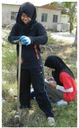
Figure 2: Soil sampling process using hand auger
