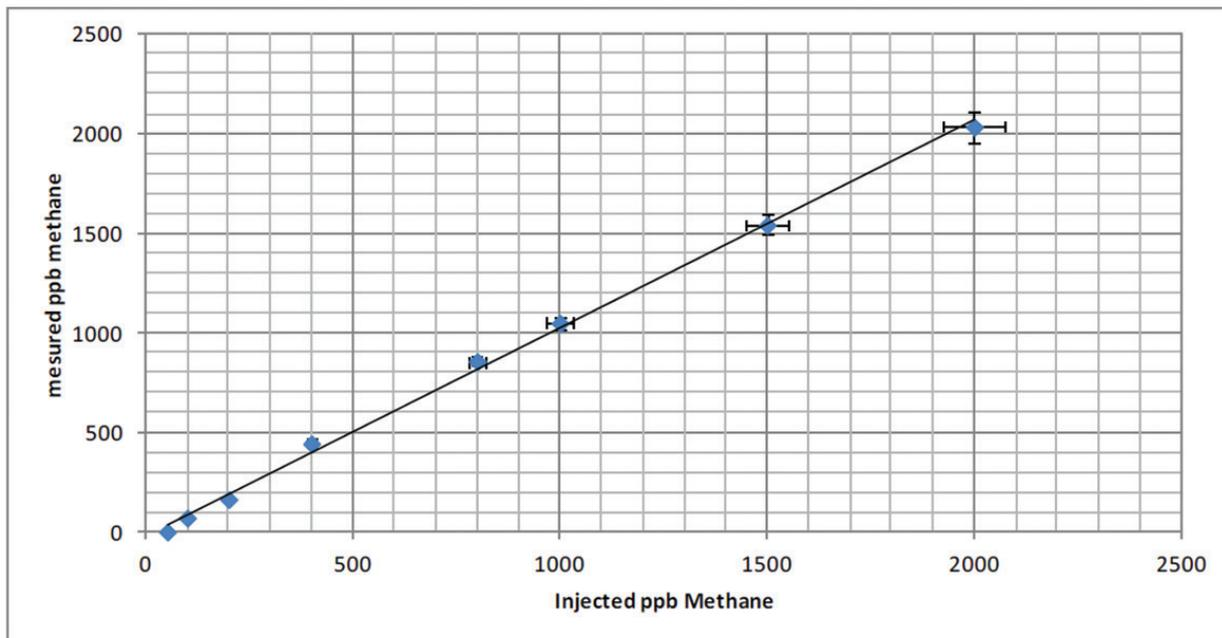
Figure 2. Linearity curve for methane using high amplification
