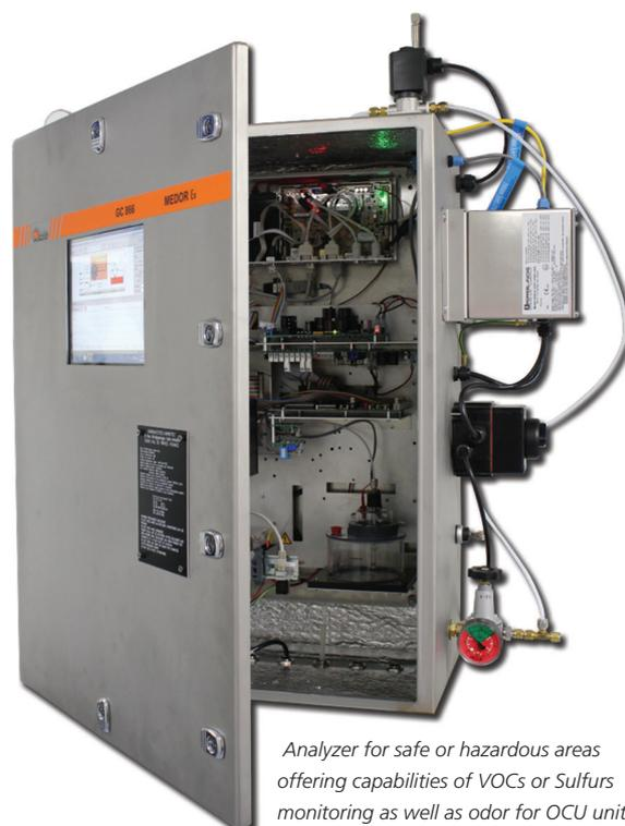
Analyzer for safe or hazardous areas offering capabilities of VOCs or Sulfurs monitoring as well as odor for OCU units
