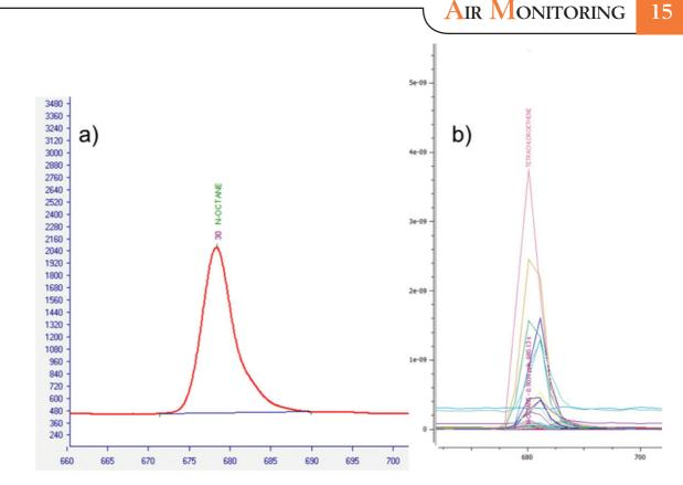
Figure 1. Chromatograms, intensity of the signal [A] vs. retention time (s), of the N-Octane and tetrachloroethene coelution observed by FID detection (a) solved with the MS (b) for C6-C16 analysis.
