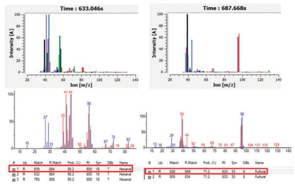
Figure 2. Automatic comparison between mass spectra obtained (top) and reference (bottom).
