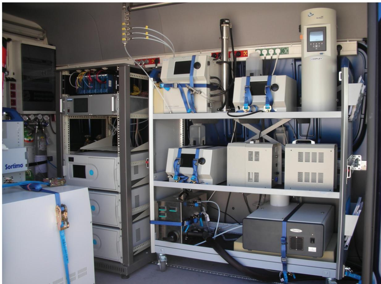
The van interior is fitted with analysers for both engine emissions monitoring and ambient air quality
